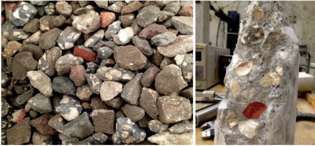
Fig. 1—Recycled construction debris used as coarse aggregate (left) in concrete (right).
